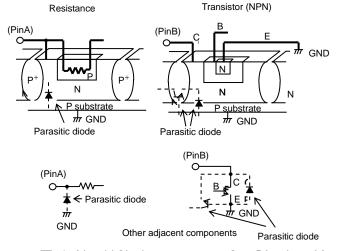
図-1 Simplified structure of a Bipolar IC
