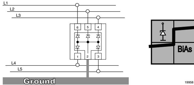
b. If symmetrical clamping behaviour is required the VESD05A5A-HSF can also be used as a bidirectional symmetrical protection device protecting up to 4 lines. In this case pin no. 2 must not be connected.
