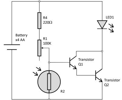
The circuit operation is very simple. When the input to the transistor Q1, which is fed from the connecting point of R1 and R2, is greater than 1.4V the output (LED), is turned on. The voltage at the join of R1 and R2 is determined by the ratio of the two resistors. This is known as potential divider.
