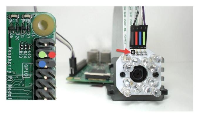
On the picture above you will see a square black mark on the PCB. That is the GND pin 1, which connects to physical pin 6 on the Raspberry Pi. Connect the other wires according to the colour coding in the picture.
