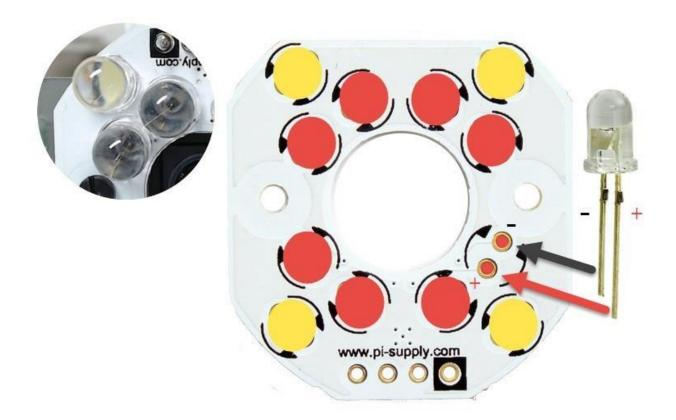
The cathode of the LEDs (short leg) needs to be on the same side as the arrows point to on the PCB. As noted above, the four LEDs in a separate bag are the bright white ones, these are intended to go in the four corner spots around the edge (bottom left, top left, top right, bottom right). All of the other 8 LED locations should be filled with the IR LEDs. We would recommend soldering the IR LEDs first (as they are in the centre) and then the white ones around the edge last.
