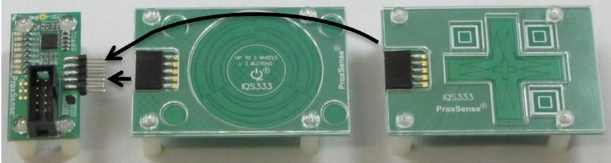
Figure 1 Connection board (left), Wheel board (middle) and Cross board (right)
