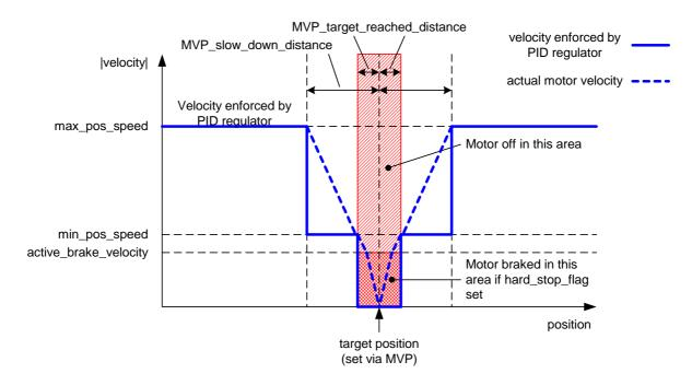
Figure 5.2: Parameterizing the positioning algorithm
