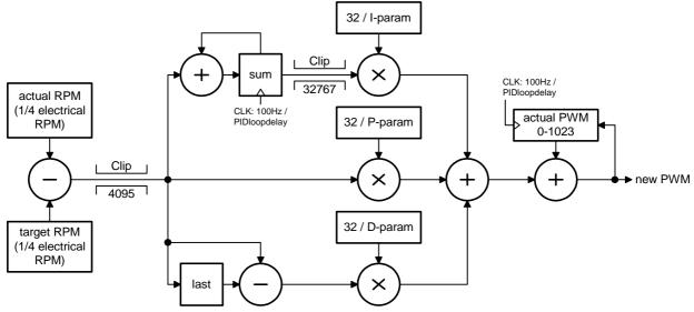
Figure 5.1: PID velocity regulator parameters
