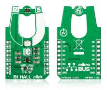
BI HALL click<sup>™</sup> is a simple solution for adding a bipolar Hall switch to your design. It carries the Melexis US2882 bipolar Hall-effect switch and a 74LVC1T45 single bit, dual supply transceiver. BI HALL click<sup>™</sup> communicates with the target board through the mikroBUS<sup>™</sup> INT line. The board is designed to use either a 3.3V or 5V power supply (which also defines the logic level of the output signal).
