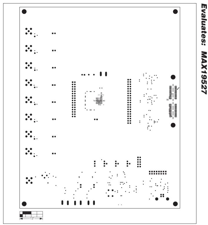
Figure 14. MAX19527 EV Kit PCB Component Placement Guide—Solder Side
