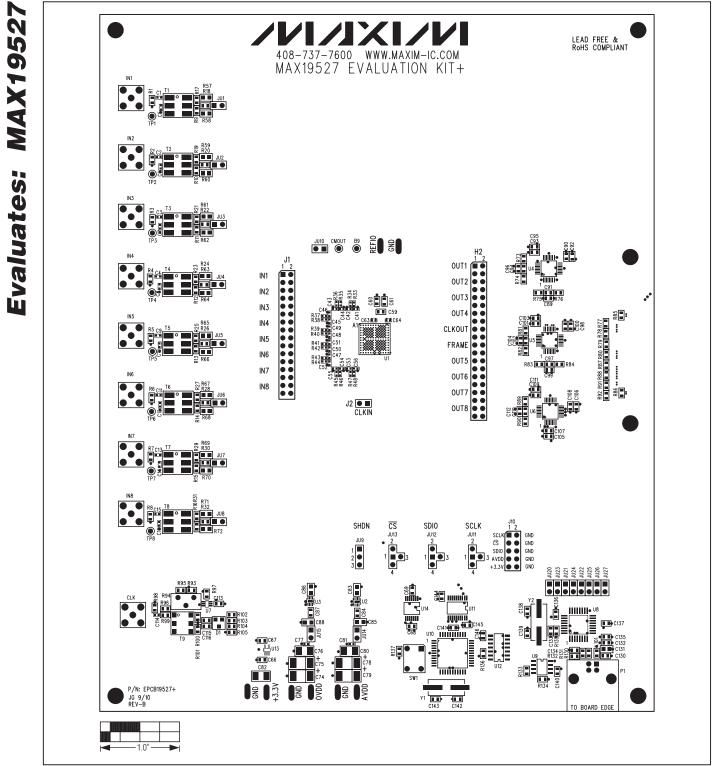
Figure 7. MAX19527 EV Kit Component Placement Guide—Component Side
