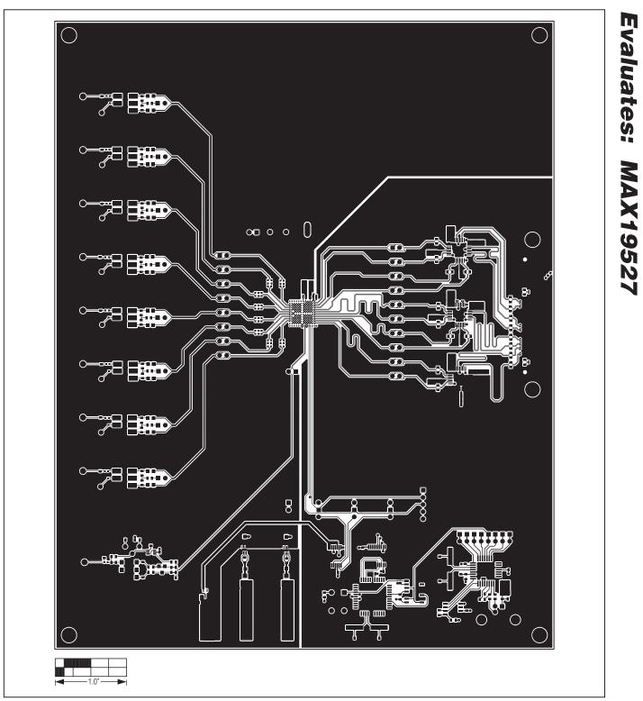
Figure 8. MAX19527 EV Kit PCB Layout—Component Side
