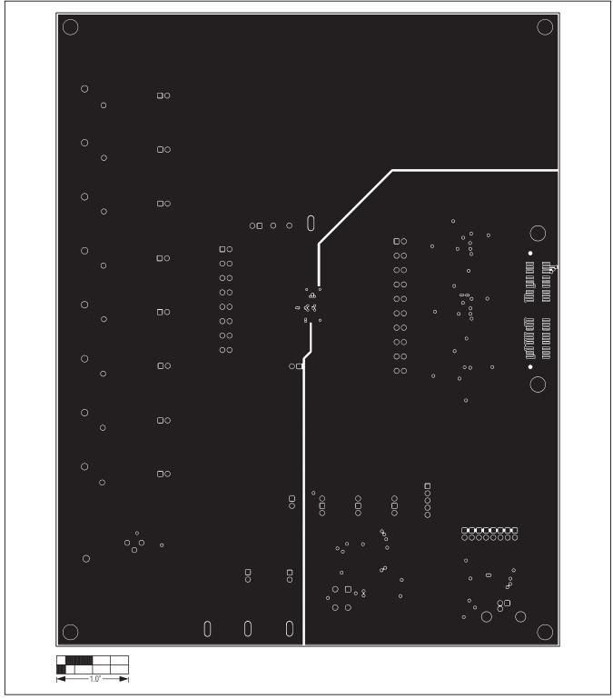
Figure 13. MAX19527 EV Kit PCB Layout—Solder Side
