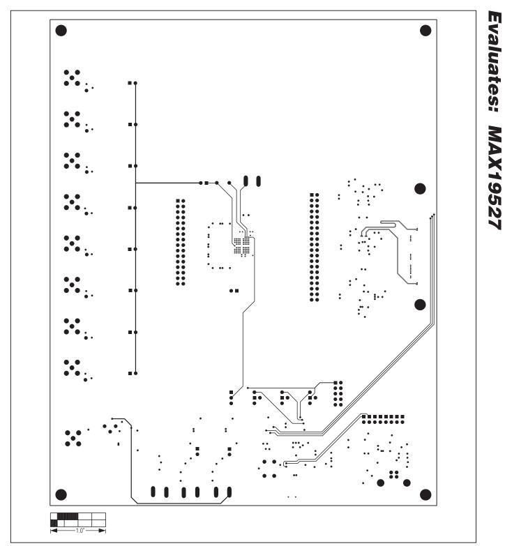
Figure 12. MAX19527 EV Kit PCB Layout (Inner Layer 5)—Routing Plane
