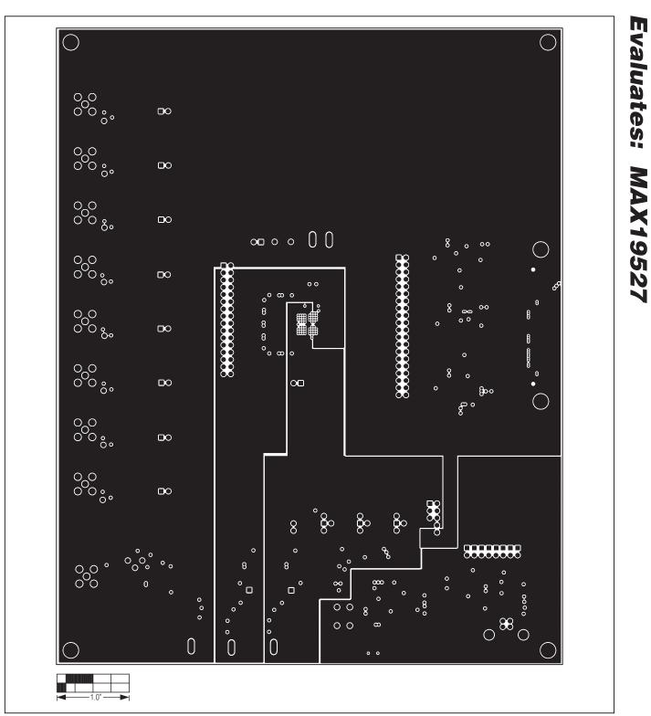
Figure 10. MAX19527 EV Kit PCB Layout (Inner Layer 3)—Power Planes
