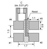
To maintain stable operation, provide a 0.01 $\mu$ F to 0.1 $\mu$ F by-pass capacitor at a location as near as possible to the power source terminal of the crystal product (between Vcc - GND).
