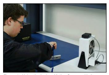
Figure 4. Using the Ionizer Motion Sensor with the 60505 High Output Bench Top Ionizer
