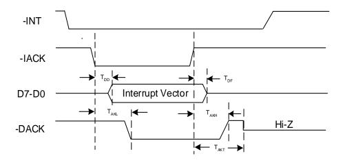
Figure 7: Interrupt Timing
