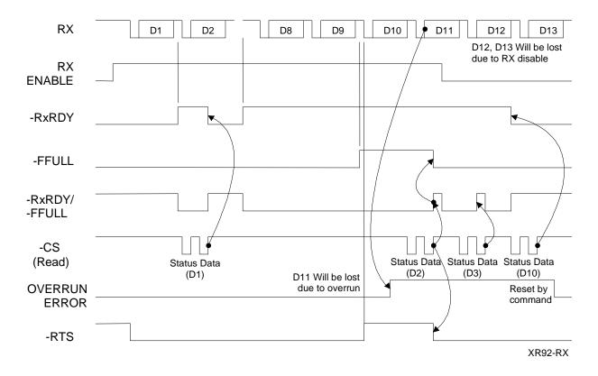
**Figure 8: Receive Timing**
