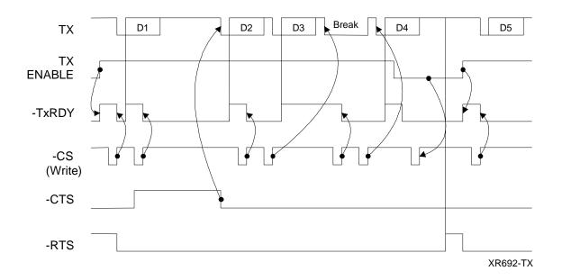
Figure 9: Transmit Timing
