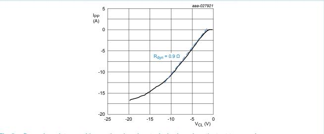
Fig. 5. Dynamic resistance with negative clamping; typical values; Input/output to ground
