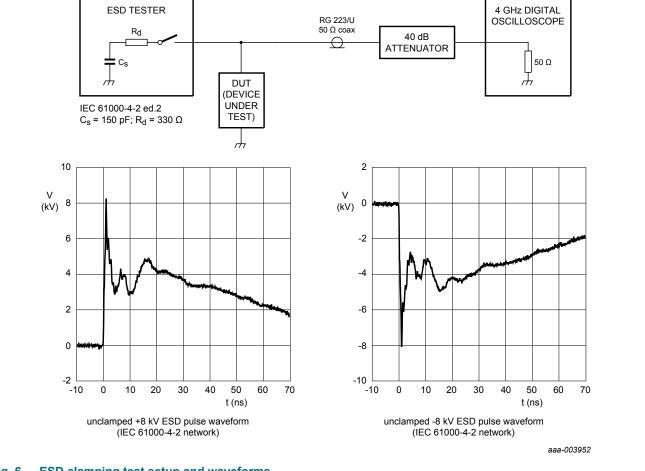
Fig. 6. ESD clamping test setup and waveforms
