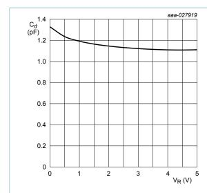
Fig. 3. Input/output to ground capacitance as a function of reverse voltage
