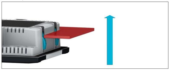
3) Please make sure to insert the device carefully into the switching cabinet. After that, the tensioners will snap back to the front. Now, the device is safely fixed in the installation recess.
