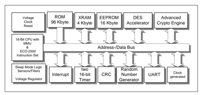
Figure 2: Block Diagram SLE 66CX162PE
