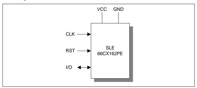
Figure 1: Pin Configuration
