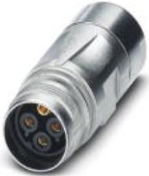
Coupler connector, straight, SPEEDCON locking, M17, Number of positions: 3+PE, Type of contact: Socket, Crimp connection, shielded: yes, Cable diameter: 5 mm...9.2 mm
