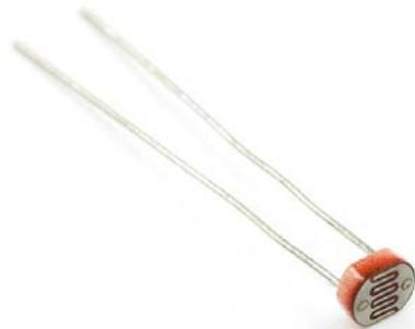
The photoresistor changes its resistance based on the light to which it is exposed. To use this with the RedBoard, you will need to build a voltage divider with a 10K Ohm resistor as shown in the wiring diagram for this experiment. The 101 board cannot read a change in resistance, only a change in voltage. A voltage divider allows you to translate a change in resistance to a corresponding voltage value.
