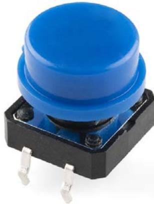
A momentary push button closes or completes the circuit only while it is being pressed. The button has four pins, which are broken out into two sets of two pins. When you press down on the button and get a nice “click,” the button bridges the two sets of pins and allows current to flow through the circuit.
