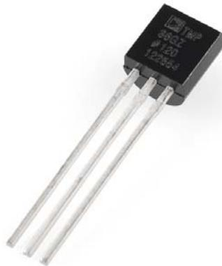
The TMP36 is a low-voltage, precision centigrade temperature sensor. It provides a voltage output that is linearly proportional to the Celsius temperature. It also doesn't require any external calibration to provide
