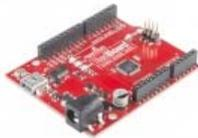
**SparkFun RedBoard - Programmed with Arduino**
