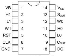
14-Pin DIP (300-mil) See Mech. Drawings Section
