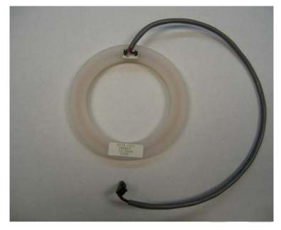
The area of the antenna is an important factor in the range the system can achieve. There is always a trade-off between available area and range required. In addition, the area the transponder antenna encloses also affects the system range. This antenna attempts to achieve a compromise suitable for a simple system. However, this only serves as a guideline reference and is not the ultimate form factor for an antenna.
