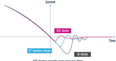
SiC diodes provide zero recovery time with negligible switching losses
