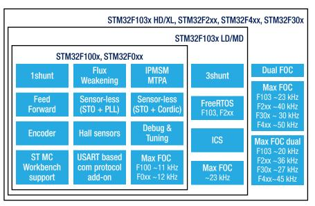
The STM3210B-MCKIT motor control starter kit comes ready-to-run with a PMSM motor or an AC induction motor (accessory). You can modify the demonstration application and develop your own motor control applications using the dedicated software libraries provided in the starter kit in conjunction with a third-party IDE and C compiler.
