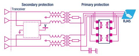
The diagram shows the use of the SLVU2.8-4A1, implementing 10/100 Mbit/s Ethernet protection.
