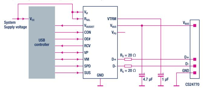
The STUSB03E is a single-chip transceiver that complies with the physical layer specifications of the Universal Serial Bus (USB) v2.0 standard. It has an integrated 5 V to 3.3 V regulator which allows direct powering from  $V_{BUS}$ . The transceiver has an integrated voltage detector to detect the presence of  $V_{RUS}$  and features an internal D+ pull-up resistor implemented in accordance with the 27% resistor ECN.
