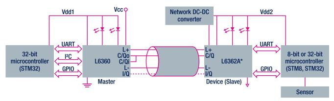
Using our MultiPower BCD technology that allows the design of the logic part, and robust LV power MOSFETs in the same chip, ST offers an efficient, compact and cost-effective solution to drive any 3-wire digital sensor.
