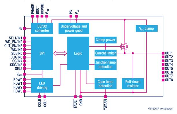
IPS devices are designed to safely drive every kind of load in low-voltage applications (up to 55 V), handling data in and out of the microcontroller by means of status/input signals. IPS devices are designed to comply with the following international standards:
