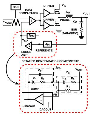
FIGURE 7. VOLTAGE-MODE BUCK CONVERTER COMPENSATION DESIGN
