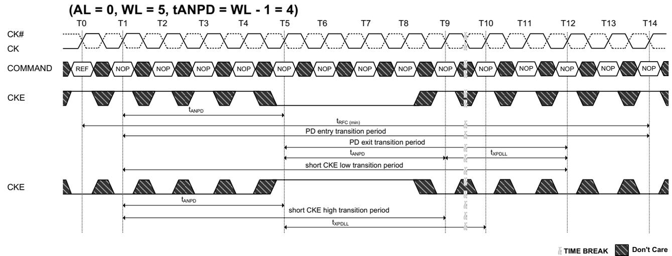
**Figure 77. Power-Down Entry, Exit Clarifications-Case 1**
