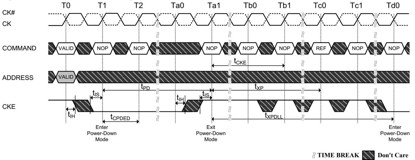
**Figure 79. Power-Down Entry,Exit Clarifications-Case 3**
