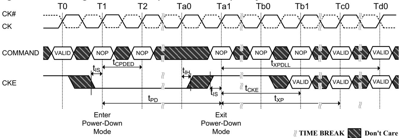
**Figure 61. Refresh Command to Power-Down Entry**
