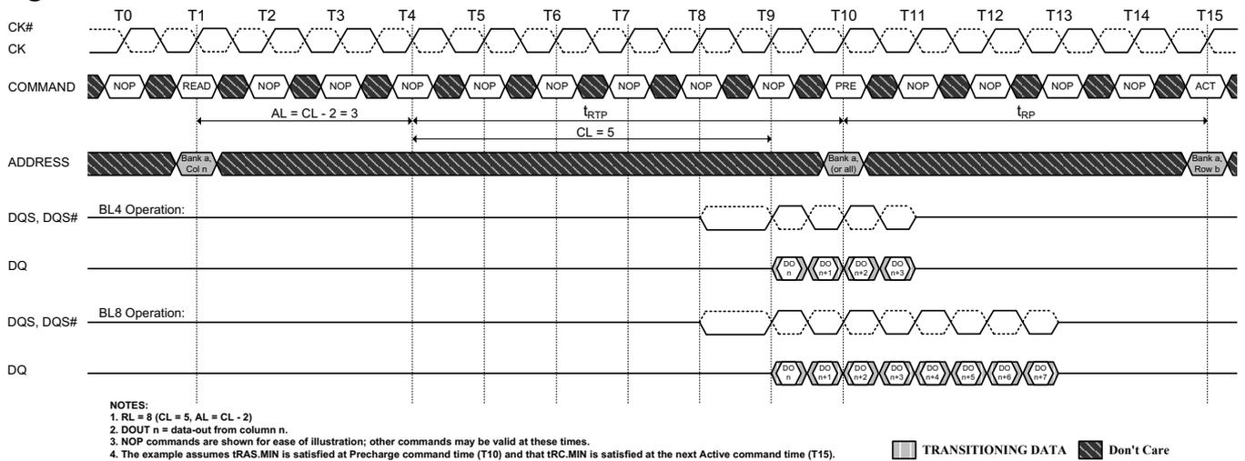
**Figure 40. Write Timing Definition and parameters**
