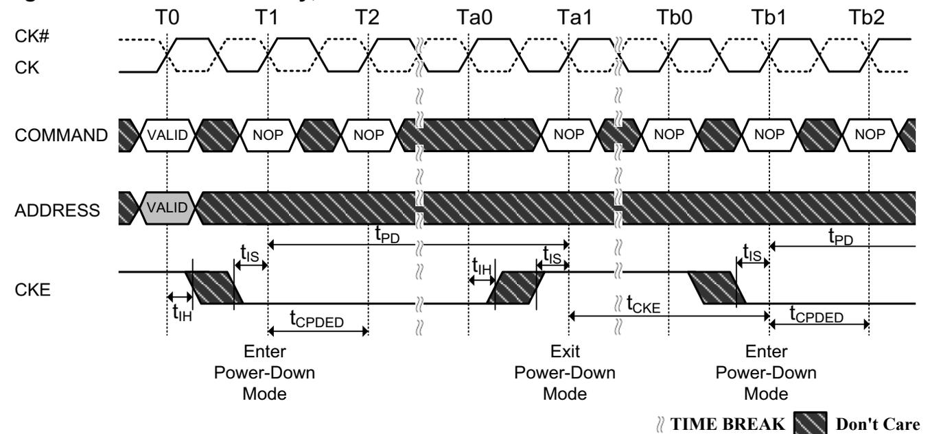
**Figure 78. Power-Down Entry,Exit Clarifications-Case 2**
