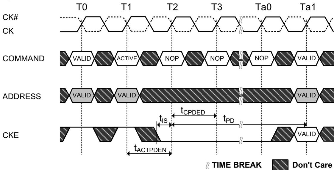
**Figure 63. Precharge, Precharge all command to Power-Down Entry**
