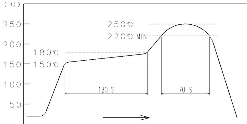
**FIG – 1 RESISTANCE TO SOLDERING HEAT
