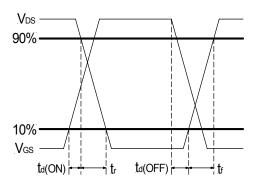
Fig. 18: switching time waveforms
