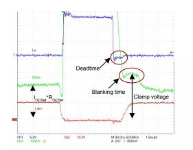
Fig. 9: OCset pin during normal condition Ch1: Inductor point, Ch2:Ldrv, Ch3:OCSet
