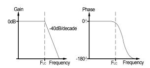
Fig. 13: Gain and Phase of LC filter
