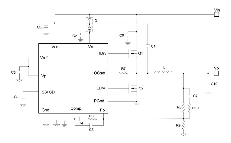
Fig.16: Application circuit for 12V to 0.9V Using ceramic output capacitor with typeIII compensation
