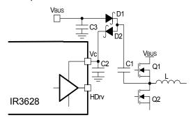
Fig. 11: Charge pump circuit to generate Vc voltage
