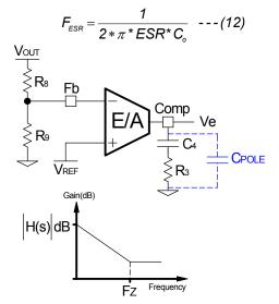
Fig. 14: TypeII compensation network and its asymptotic gain plot
