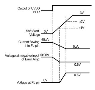
Fig. 6: Theoretical operation waveforms during soft-start
