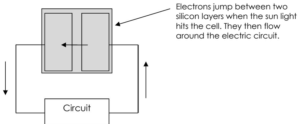
The sun generates a lot of energy but not all of this can be converted into electricity by the solar cell. The amount of the sun's energy that can be converted into energy is determined by the efficiency of the solar cell. A typical solar cell may have an efficiency of 12%. This means that if 100 Watts of light energy fell on a solar cell it would generate 12 Watts of electrical energy.
