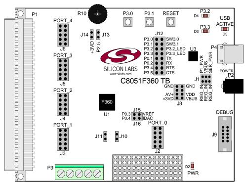
Figure 3. C8051F360 Target Board
