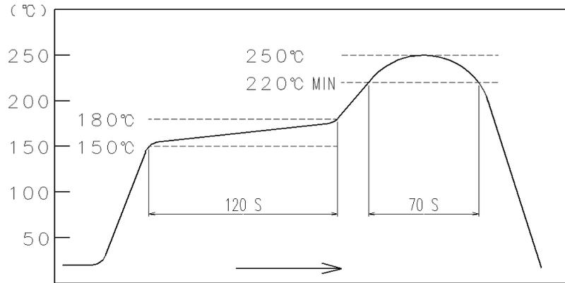
**FIG - 1 RESISTANCE TO SOLDERING HEAT
