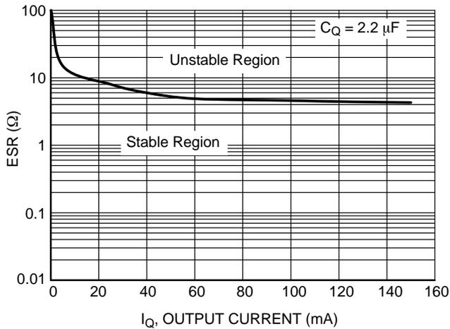
Figure 16. Output Capacitor ESR vs. Output Current
