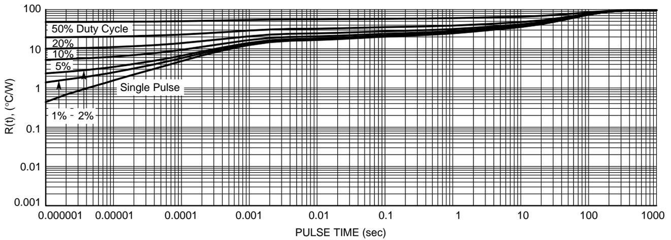
**Figure 21. Transient Thermal Response (SOIC-8 Fused)
