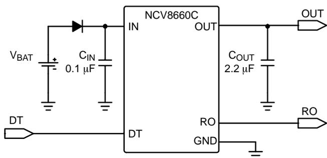
Figure 1. Application Diagram
