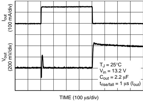
Figure 12. Load Transient
