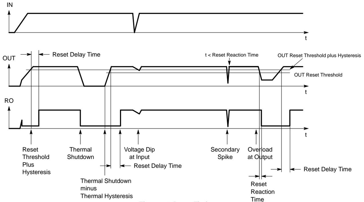
**Figure 19. Reset Timing**
