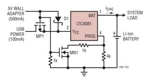
Figure 3. Combining Wall Adapter and USB Power
