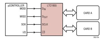
Figure 4. Microcontroller Interface
