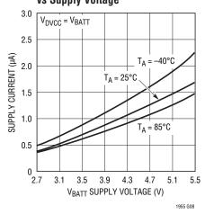
DV<sub>CC</sub> Shutdown Current vs Supply Voltage
