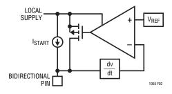
Figure 2. Dynamic Pull-Up Current Sources
