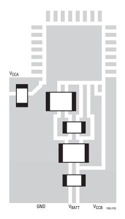
Figure 3. Optimum Single-Layer PCB Layout
