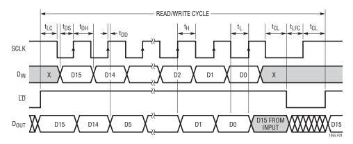
Figure 1. Serial Port Timing Diagram
