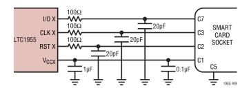
Figure 8. Additional Components for Improved Compliance Testing
