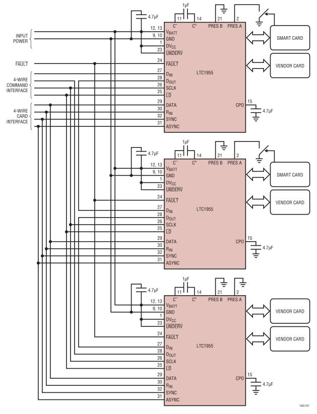
Figure 6. Multiple LTC1955s Daisychained Together
