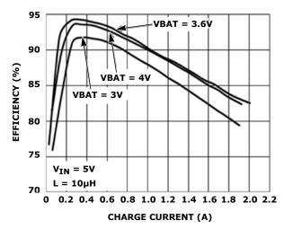
FIGURE 7. EFFICIENCY vs LOAD
