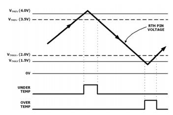
FIGURE 3. THRESHOLD VOLTAGES FOR 0°C to +50°C WINDOW ( $V_{BIAS} = 5.0V$ )
