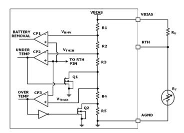
FIGURE 2. THERMISTOR INTERNAL CIRCUIT
