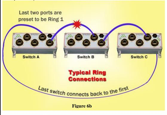
With the break indicated above, we would expect these values from the Modbus registers of each switch:
