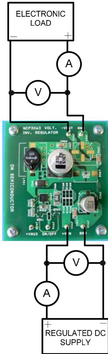
Figure 1: Test Setup DFN
