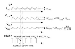
Figure 2. MIC24056 Control Loop Timing
