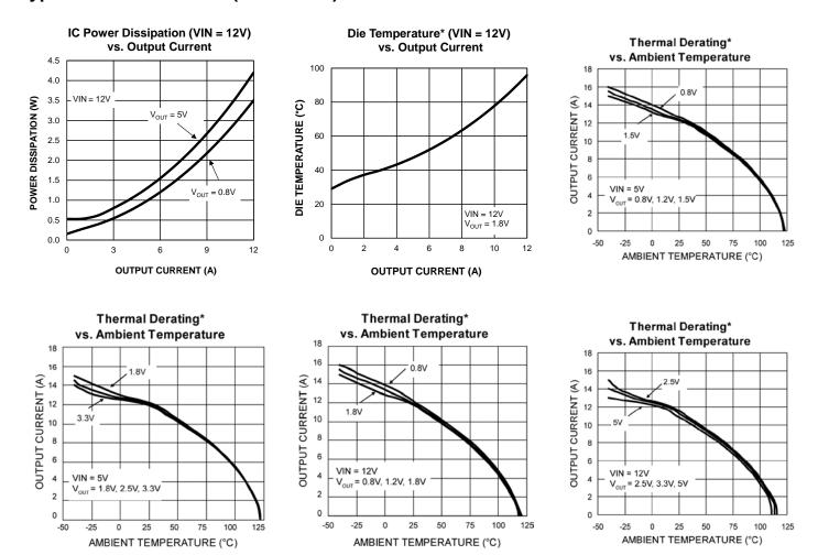
**Die Temperature\***: The temperature measurement was taken at the hottest point on the MIC24056 case mounted on a 5 square inch 4 layer, 0.62 inch, FR-4 PCB with 2oz finish copper weight per layer; see Thermal Measurement section. Actual results will depend upon the size of the PCB, ambient temperature and proximity to other heat emitting components.
