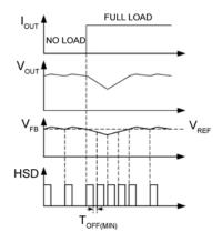
Figure 3. MIC24056 Load Transient Response
