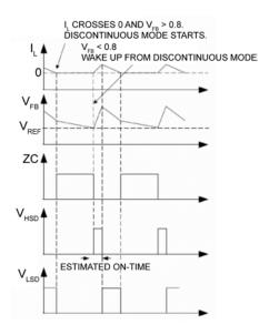
Figure 4. MIC24056 Control Loop Timing (Discontinuous Mode)
