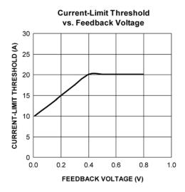
Figure 5. MIC24056 Current-Limit Foldback Characteristic
