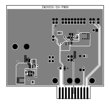
Figure 16. MIC24056 Evaluation Board Bottom Layer
