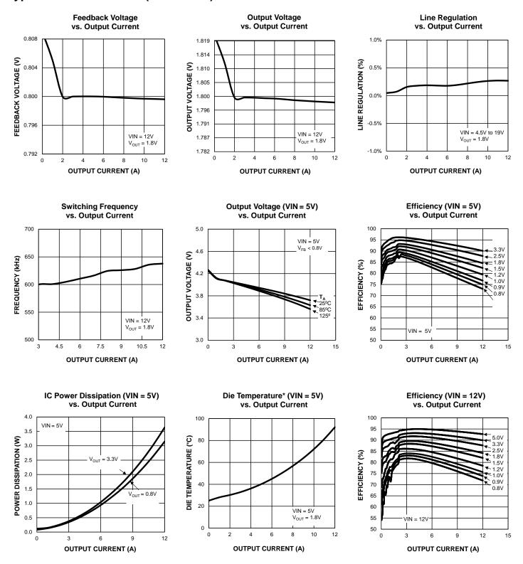
**Die Temperature\***: The temperature measurement was taken at the hottest point on the MIC24056 case mounted on a 5 square inch 4 layer, 0.62 inch, FR-4 PCB with 2oz finish copper weight per layer; see Thermal Measurement section. Actual results will depend upon the size of the PCB, ambient temperature and proximity to other heat emitting components.
