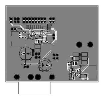
Figure 15. MIC24056 Evaluation Board Mid-Layer 2
