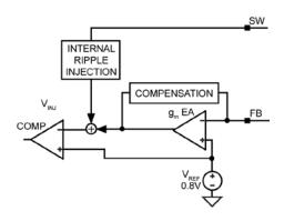
Figure 10. Internal Ripple Injection
