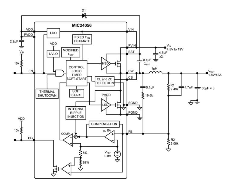
Figure 1. MIC24056 Block Diagram
