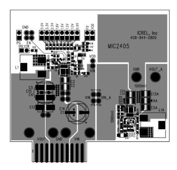
Figure 13. MIC24056 Evaluation Board Top Layer
