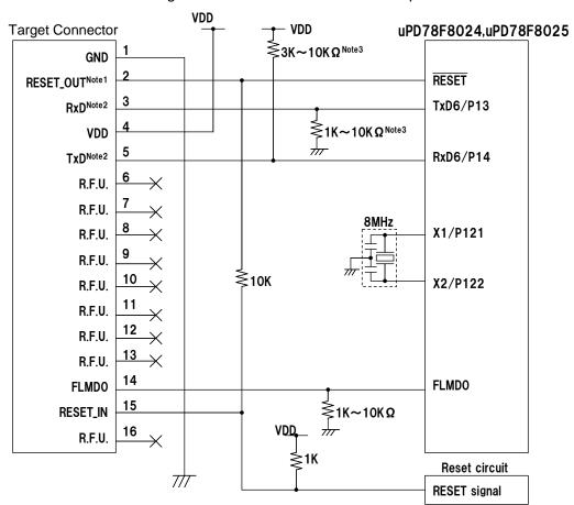
Figure 3-2 Circuit Connection Example
