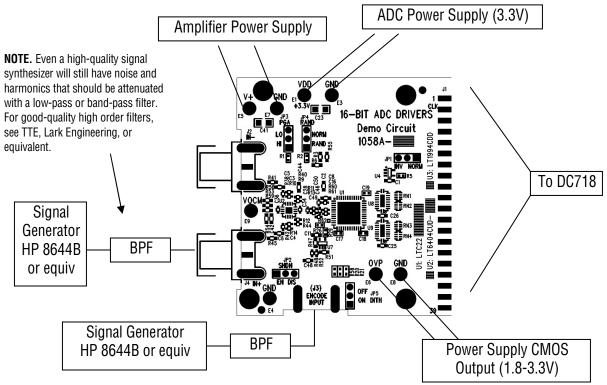
Figure 1. Proper Evaluation Equipment Setup
