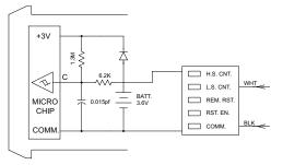
Moving the white wire to the "H.S. CNT." Input allows the CUB Counter to operate at speeds up to 5 KHz when driven by bi-polar outputs or external circuits having an output impedance of 3.3 K $\Omega$  or less. Input drive voltage must be limited to 3.0 V maximum to avoid damage to the counter. Outputs higher than 3.0 V can be used with an external voltage divider, as shown.
