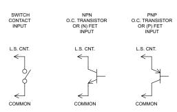
Reed switches, mercury wetted contacts, snap action limit switches, and silver alloy relay contacts with wiping action are usually satisfactory for generating count input signals. Motor starter contacts, tungsten contacts, and brush-type contacts should **NOT** be used. Normally open contacts are recommended for longer battery life and greater noise immunity.
