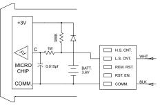
Pulling the "L.S. CNT." Input to Common with a mechanical or solid-state switch increments the counter. The low pass filter (1 meg resistor and 0.015 pf cap) used with a Schmidt trigger circuit debounces mechanical switch signals. The switch load is  $14 \mu A$  (max. voltage drop 0.5 V) when ON. OFF-state leakage current must be less than  $2 \mu A$ .
