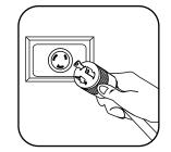
AC Input Connection: Insert L5-20P twist-lock plug into compatible L5-20R utility, generator or UPS outlet. (Included adapter converts L5-20P to 5-20P for connection to 5-15/20R outlet.)
