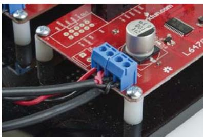
It's generally a good idea to hook up the power to the RedBoard and logic circuitry before you power the AutoDrivers; do note that you can't access the AutoDriver boards via SPI until BOTH parts are powered, however.
