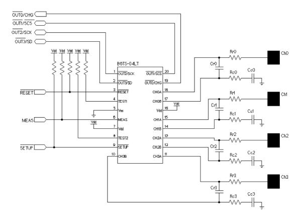
Note 1: Connect Rr, Cr, Rc, and Cc to each touch electrode, as shown in the above figure. Refer to the design tool (B6TWWorkbench) for their actual values.
