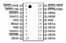
Note 1: Pins TEST1, and TEST2 are used for testing during manufacture of the IC. When using these pins, connect them to VDD through a pull-up resistor.
