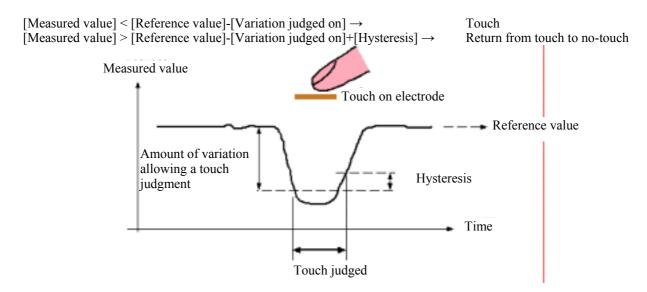
Even in the touched state, the measured value changes according to variation in the environment (output drift). The chip is provided with an automatic drift-correction function, which can cancel mild changes of the measured value due to variation in the environment (drift correction function).
