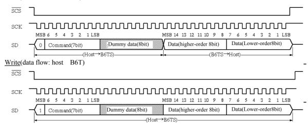
If data communication is performed during normal measurement mode, the measurement operation stops while the data is communicated.
