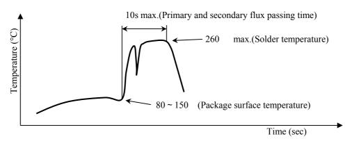
Fig.2 Wave soldering method temperature profile
