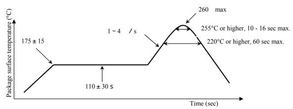
Fig.1 Reflow method temperature profile
