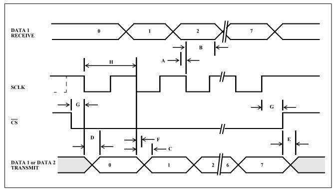
Figure 13 - Serial Microport Timing Diagram
