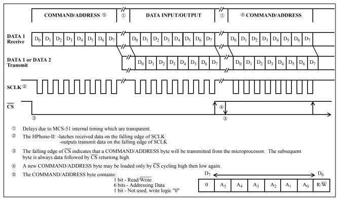
Figure 6 - Serial Port Relative Timing
