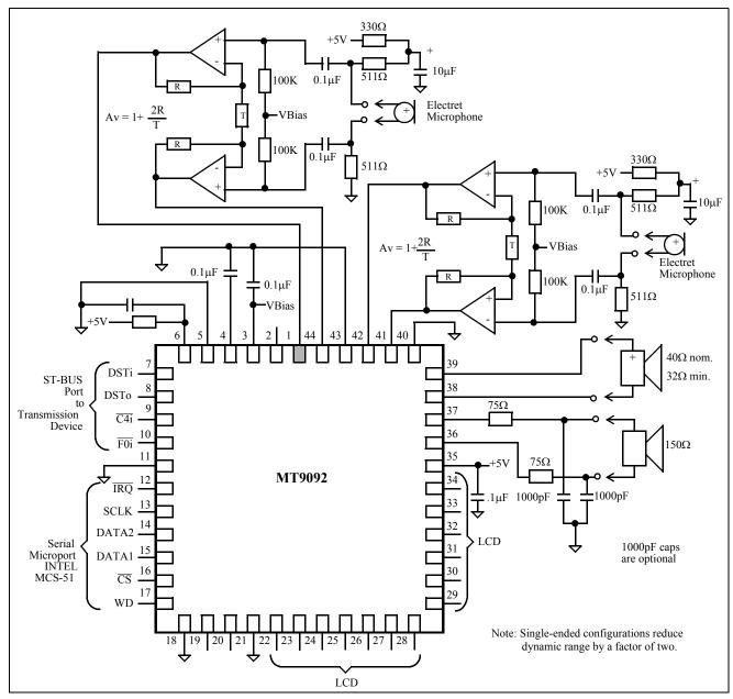
Figure 8 - Application Circuit - Fully Differential Audio Input
