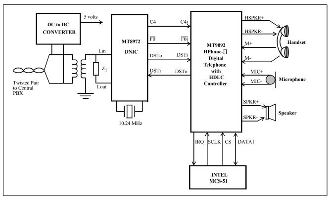
Figure 11 - Voice/Data Digital Telephone Set Circuit
