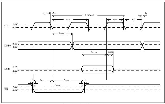
Figure 12 -ST-BUS Timing Diagram
