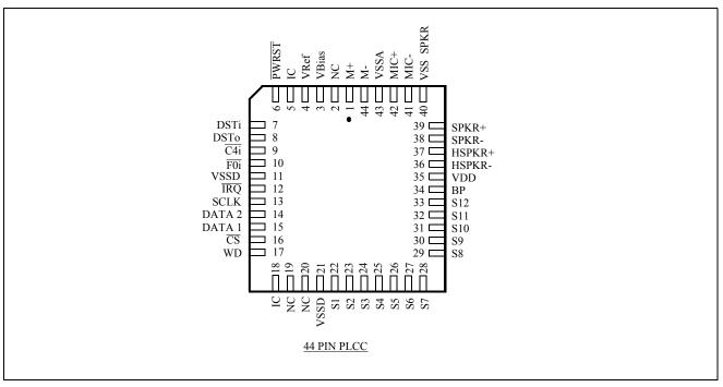
Figure 2 - Pin Connections
