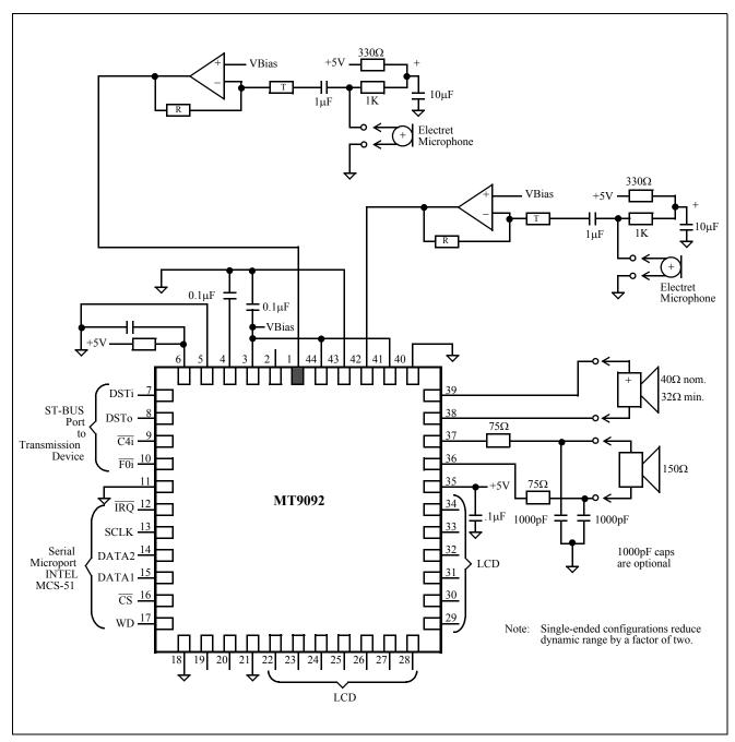
Figure 9 - Application Circuit - Single-Ended Audio Input
