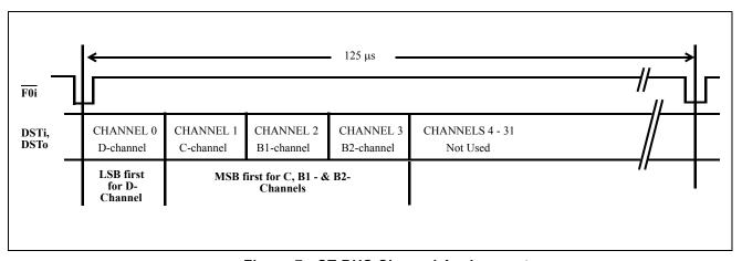
Figure 7 - ST-BUS Channel Assignment
