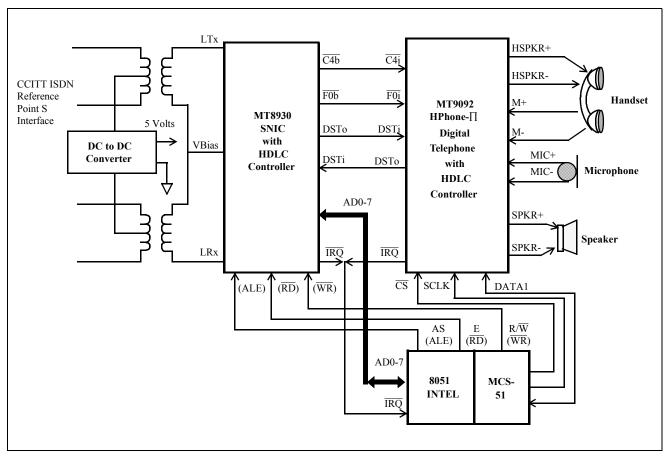
Figure 10 - CCITT ISDN Voice/Data Terminal Equipment - TE1
