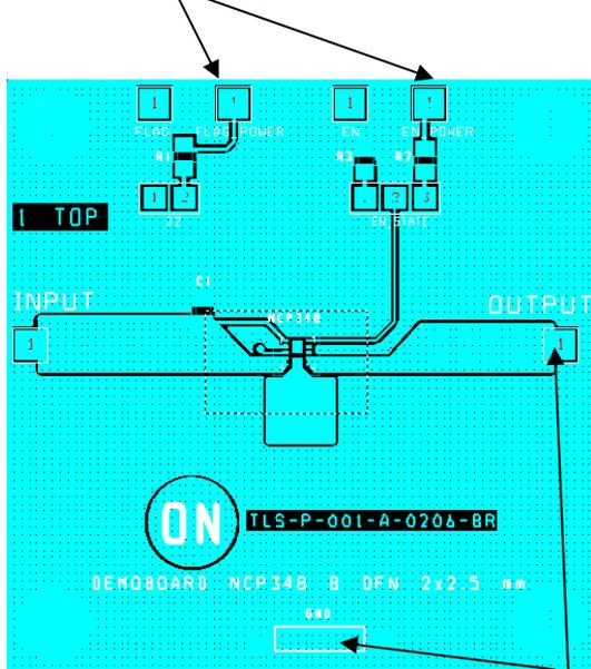
Connect 2.5 ohms load between Vout and GND.
