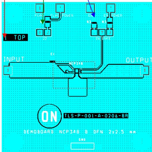
Connect +5V supply on FLAG\_POWER pin and EN\_POWER pin. (use same supply)
