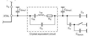
Using  $C_4$  = 8.2pF ±5%,  $C_5$  = 10pF ±5%, a switch port with  $C_{Switch}$  = 3pF ±10%, stray capacitances on each side of the crystal of  $C_{Stray2}$  = 1pF ±10%, a parallel capacitance of the crystal of  $C_0$  = 3.2pF ±10%, and a crystal with  $C_M$  = 13 fF ±10%, typically results in an FSK deviation of ±21.5kHz with worst case tolerances of ±16.25kHz to ±28.01kHz.
