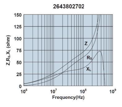
Impedance, reactance, and resistance vs. frequency.
