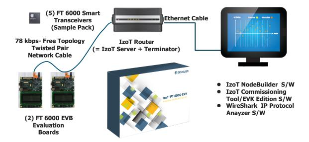
IzoT NodeBuilder software, you write your device applications using the Neuron C programming language, a high-level language based on ANSI C with extensions to simplify network communication, hardware I/O, and event-driven processing. The Neuron C language supports up to 254 address table entries, 254 static network variables and 127 network variable aliases per device for devices based on a Series 6000 chip with Neuron Firmware version 21 or newer, subject to available memory.
